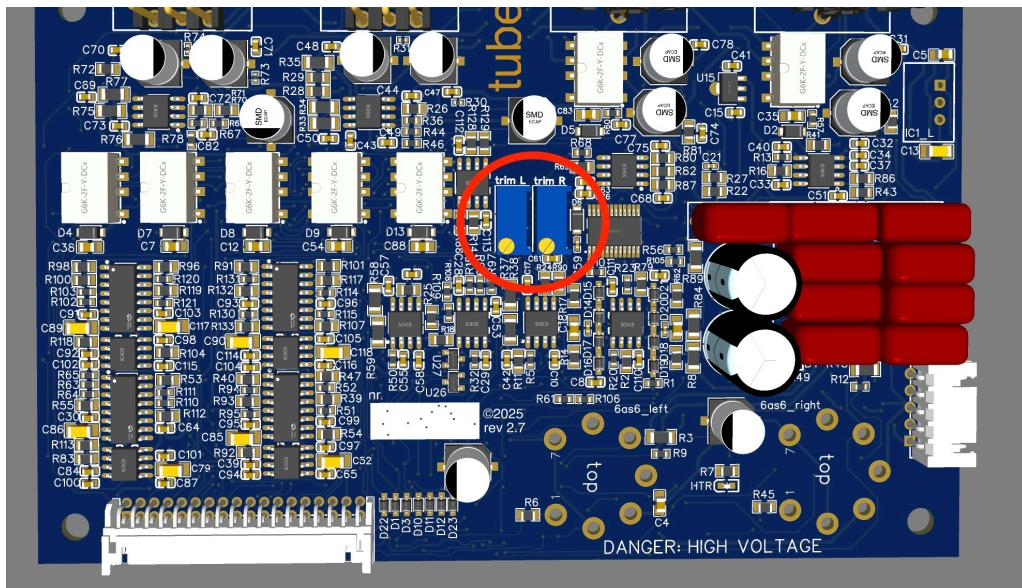
There are two trimmers in the middle of the motherboard which calibrate the output signal of the tubes by a few dB. After replacing the tubes it's best to check these and recalibrate when needed.
