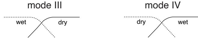
In filter mode III and IV the mix of the dry and wet output levels will determine the resulting overall frequency response. If you're looking for a flat overall frequency response, it's important to keep the dry and wet output levels in balance with each other. Easiest is to verify quickly by putting the unit in bypass.
